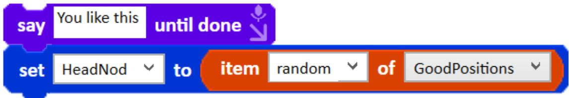
A speech block can be used to make the robot talk.
