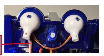
5. Replace the screws to hold the eyeballs in place
