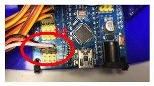
7. Connect the plug so that the white or orange wire is on the right hand side and the black or brown wire is on the left as shown.
