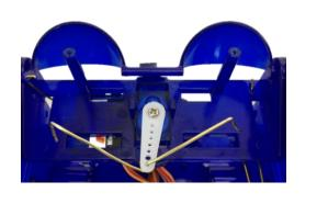
5. Put the new eyeballs in place with the wires to the bottom of the eyeball. Replace screws and bend ends of wires.
