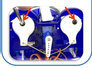
$\Im.$  Straighten the ends of the link and pull out of the holes at the back of the eyeballs
