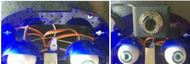
3. Plug in the camera using the supplied USB extension cable. Start the Ohbot program and select Sensor from the Settings menu. Select the camera from the list of video devices and set the resolution to 160, 120.
