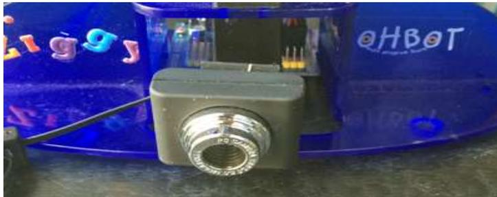
3. Plug in the camera using the supplied USB extension cable. Start the Ohbot program and select Sensor from the Settings menu. Select the camera from the list of video devices and set the resolution to 160, 120.
