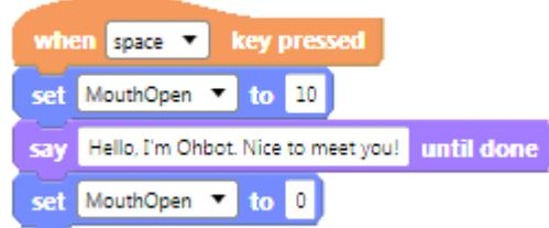
But this is not ideal since Ohbot's mouth will not open and close as the words are spoken. An alternative approach is to use the speech sensor block. This gives a value between 0 and 10 when Ohbot speaks. We can then repeatedly set the position of the mouth to this value using a forever loop.
